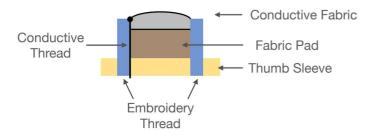
Each electrode is made of a layer of conductive fabric on top of a thick fabric pad to improve skin contact. The sensors are embroidered to an elastic fabric thumb sleeve and connected via conductive thread to the OpenBCI Cyton board for biopotential sensing [3].
