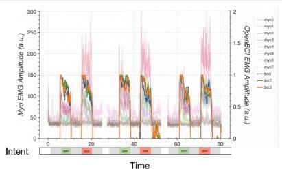
Using a bandpass filter (50 Hz to 125 Hz), preliminary testing of the fabric sEMG sensor data alongside the commercial sEMG armband in a healthy participant demonstrates its capacity as an EMG sensor for intrinsic muscle activity.
